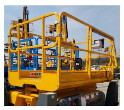
Remove platform control box from its designated position and place it on platform floor
